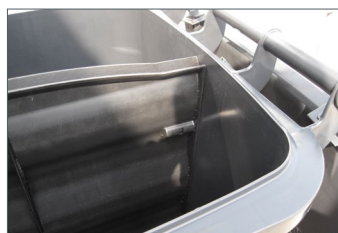
Cloison de separation
