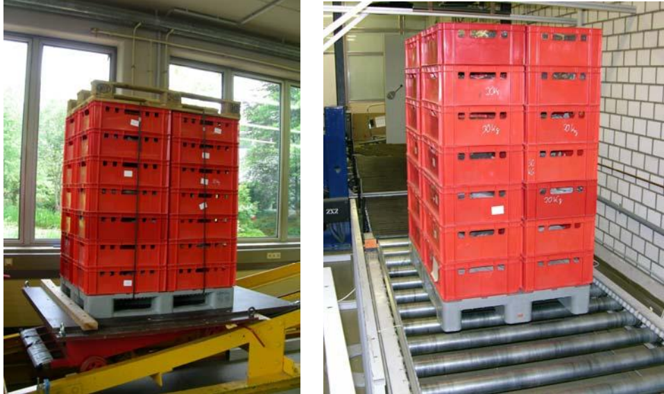
Fig. 3 and Fig. 4: Test structure: Left: Horizontal impact test: Right: Roller conveyor test
