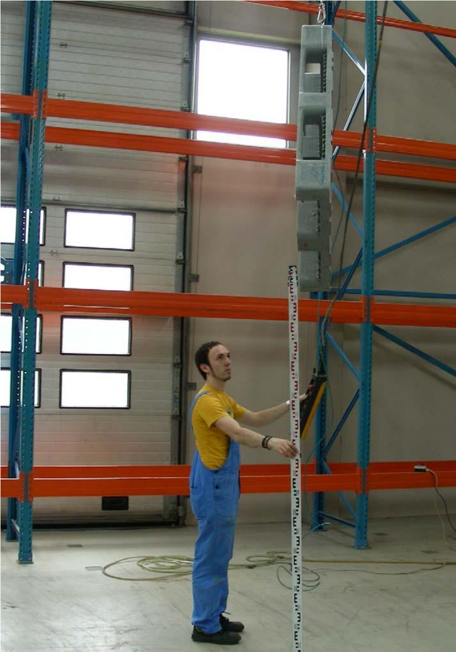
Fig. 2: Drop test following temperature conditioning
